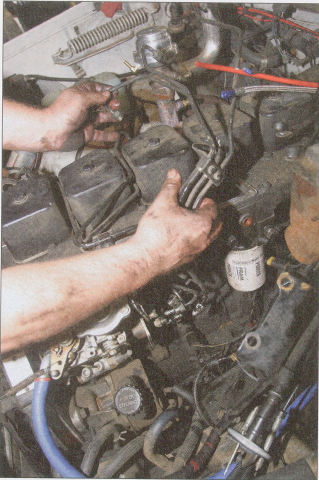
Before the Cummins cylinder head can be removed, everything else on top of it must be taken off. This means the intake horn, throttle linkage, coolant lines, and injector lines. When removing the injection lines, make sure to take them off at the pump and remove them in two pairs of three, otherwise they'll end up like spaghetti when you try to re-install them.
