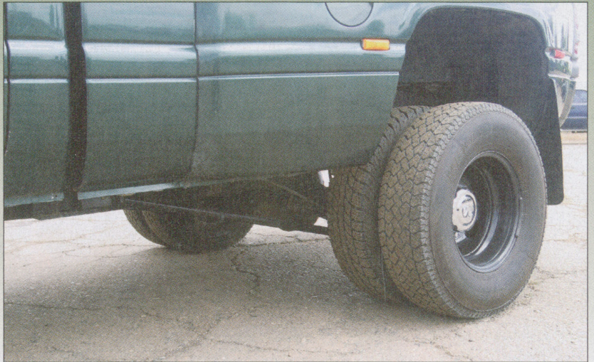
Out back, a custom set of traction bars plants the four rear tires to achieve optimum traction.
