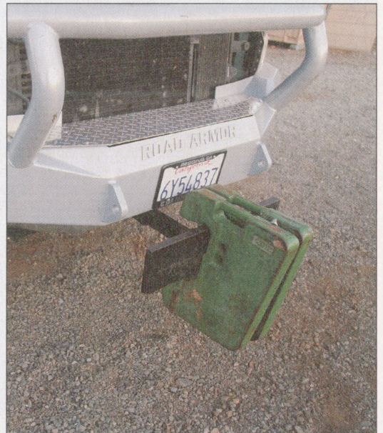
Joel hooks as many tractor weights as he can to the already heavy Road Armor bumper for utmost weight and traction. With or without the weights, the truck tips the scales at darn near 8,000 pounds.
