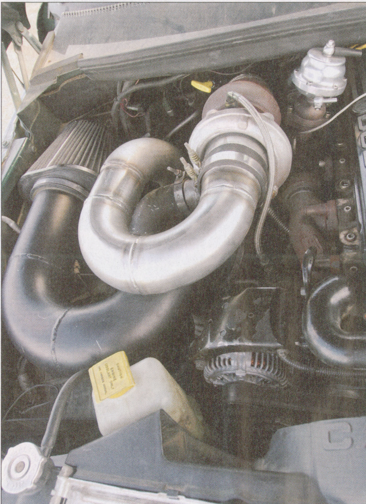
The 58mm and 74mm turbos combine to produce 70 psi of boost and limit EGT to 1,600 degrees, which actually isn't that excessive for a pulling truck.
