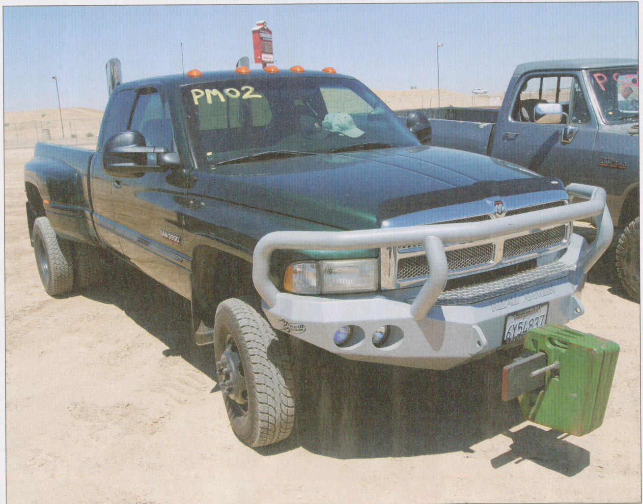
A set of Fox racing shocks smoothes out the track, so Joel's Dodge grips the pulling surface, rather than bouncing over it.
