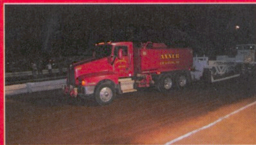
We promised you a full pull, and guess what, here it is! Weight helps traction immensely in sled pulling, and the 55,000-pound water truck was the only vehicle to make a full pull, at 302 feet.
